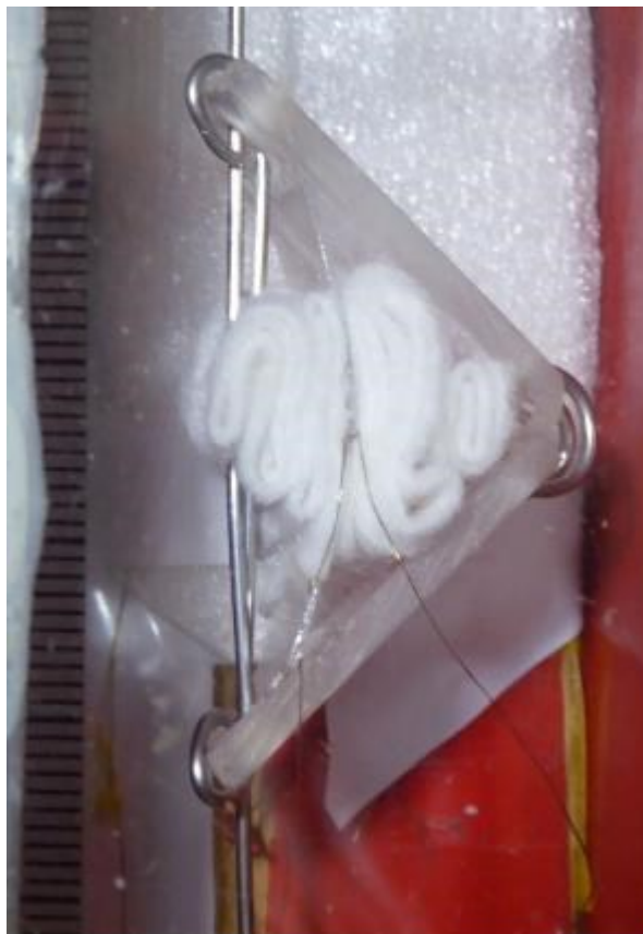
Photo 1. The hinge-shaped sample holder, ca. 30 mm high.
