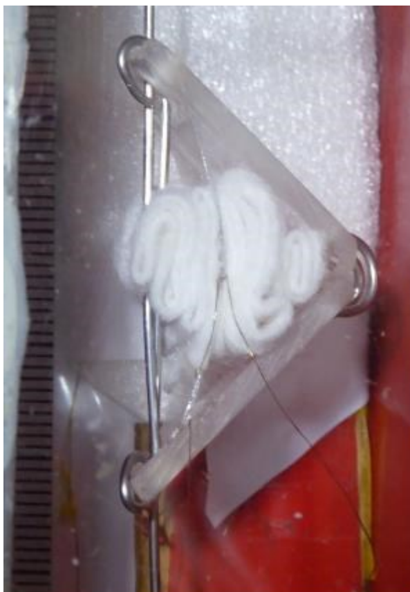
Photo 1. The hinge-shaped sample holder, ca. 30 mm high.
