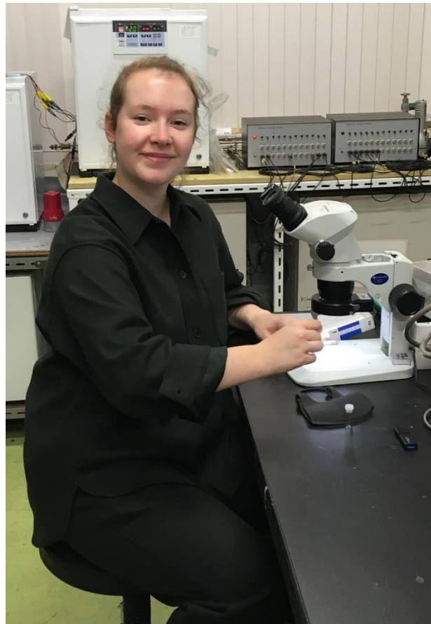
Libby (Ms. Elizabeth Kate Rusbridge) performing a sample preparation for resistivity measurement under a microscope at room G105.
